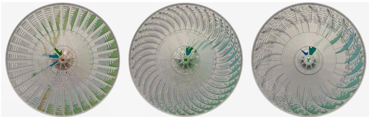
Figure 2: Optimised radial design, Vortex design, half-row double wide Vortex design DEM-SPH Simulations
