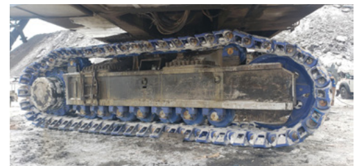
Bradken's Wide Roller Path (WRP) Installed
