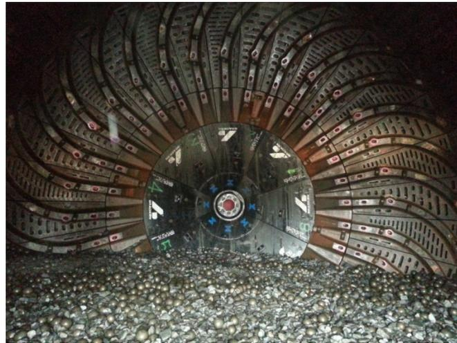
Figure 7 – Vortex discharge design installed
