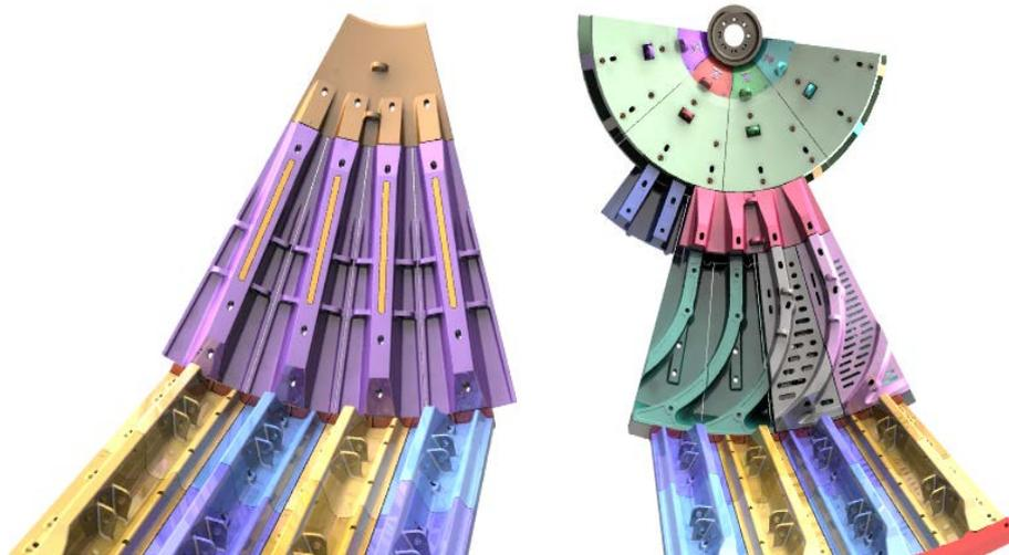
Figure 6 – General assembly of the 32ft Kansanshi SAG mill showing feed and discharge liners
