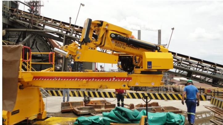
Figure 5 – The 4.5Tonne RME reline machine Installed at Kansanshi
