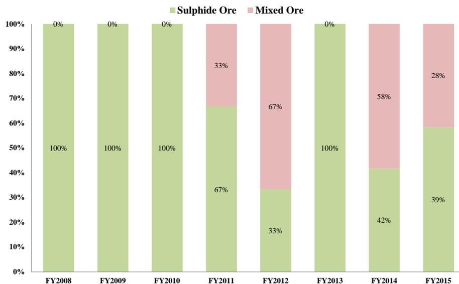
Figure 3 – Proportion of ore type processed through the 32ft SAG mill since Commissioning
