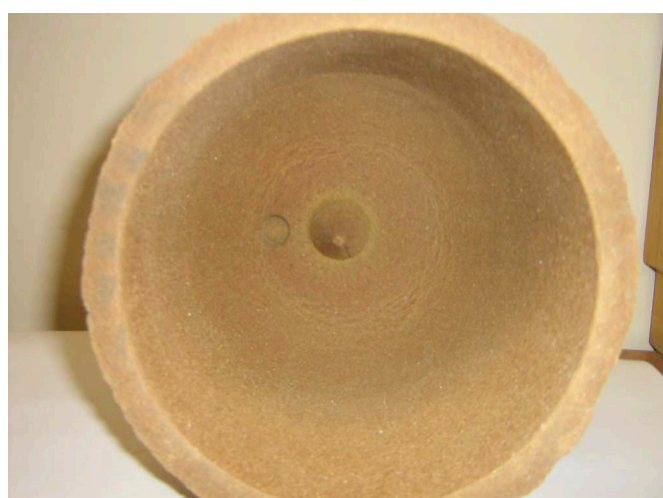
Figure 4 – Pre-shaped insulating blind riser sleeve
