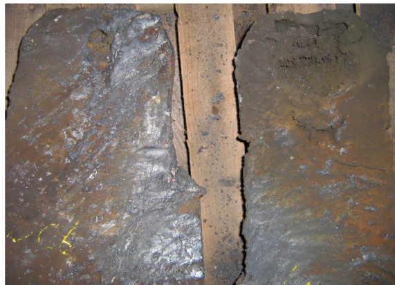
Figure 10 – The riser unassisted by a venting chamber (left) has a skin of metal formed at the top and shows an insignificant amount of metal loss. The riser assisted by a venting chamber (right) is open at the top and shows significant metal loss.
