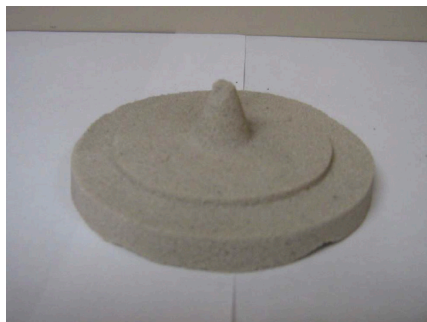
Figure 3 – Examples of sand covers for cylindrical (tube) risers
