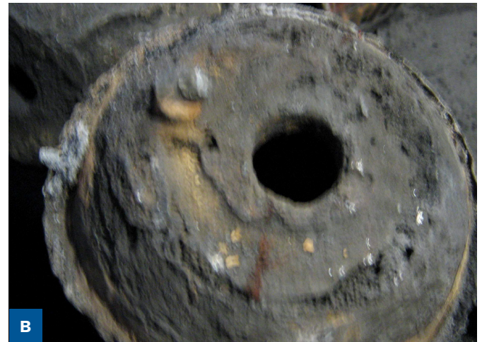
Figure 9 – (A) Blind riser moulded without a venting chamber (B) Blind riser moulded with a venting chamber
