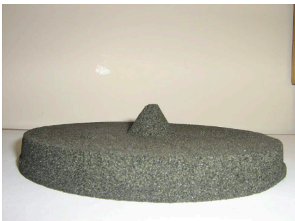
Figure 3 – Examples of sand covers for cylindrical (tube) risers
