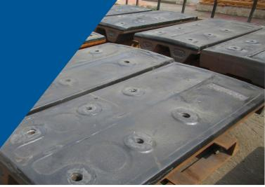
Bradken's MillSafe™ bolting system is a safe and fast solution for liner installation and removal. Install your liners by bolting them from outside your grinding mill.
