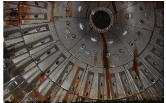
Minimal wear of the Bradken Bullnose® at 23 months
