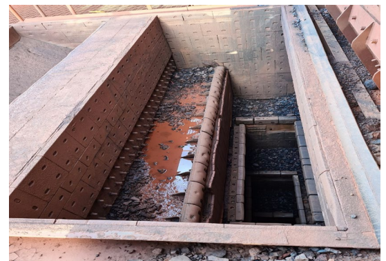
Tight area with several deep levels, making it difficult for lifting heavy liners one by one.
