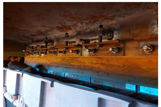
Skirt liner adjustable mountings.
