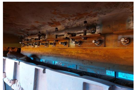
Skirt liner adjustable mountings.
