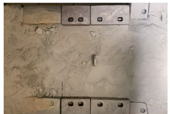
Duablock Liners used in higher wear areas
