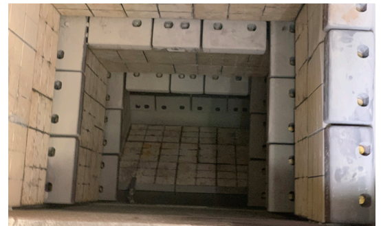
Vulcabrix liners, Duracast and Duablock Billet liners in the tripper pant legs
