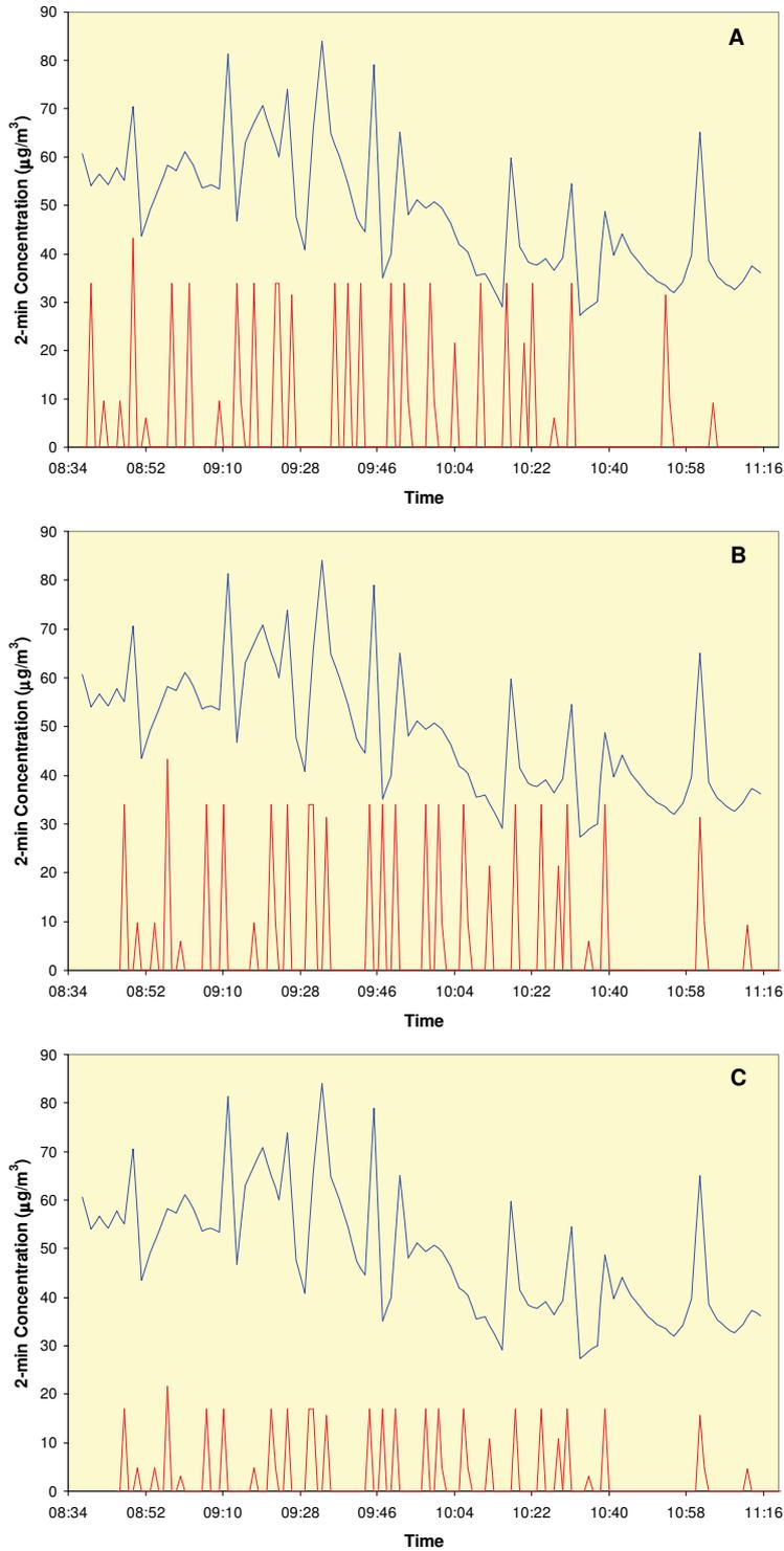
**Figure 8 Measured (blue line) and Simulated (red line) Nitrogen Oxides Concentrations at the London City Airport Newham Docklands Monitoring Site on the Morning of 15 January 2009. A = times as recorded with maxima expected aircraft contributions; B = 8 minute time shift in maxima aircraft peaks; C = 8 minute time shift in minima aircraft peaks.**
