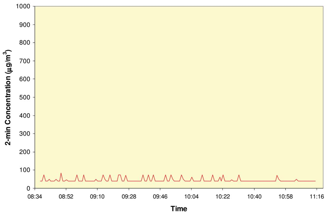
**Figure 5** Simulated Nitrogen Oxides Concentrations at the London City Airport Monitoring Site on the Morning of 15<sup>th</sup> January 2009 on a Constant Background of  $40 \mu\text{g}/\text{m}^3$
