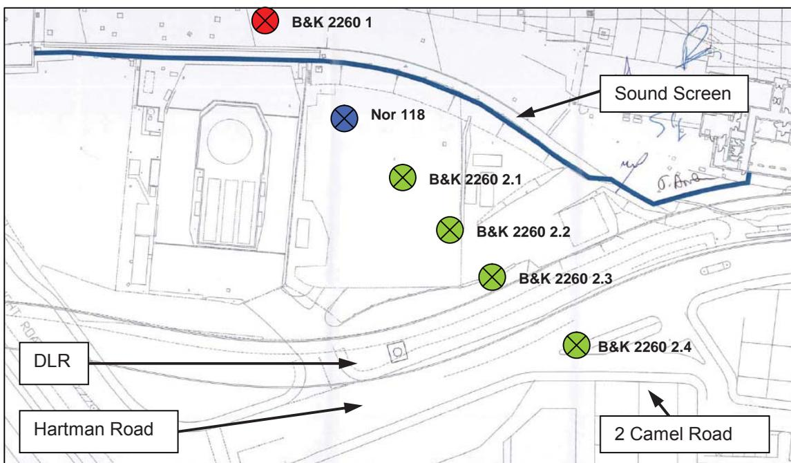
Figure 4 – Sound screen performance investigation measurement positions
