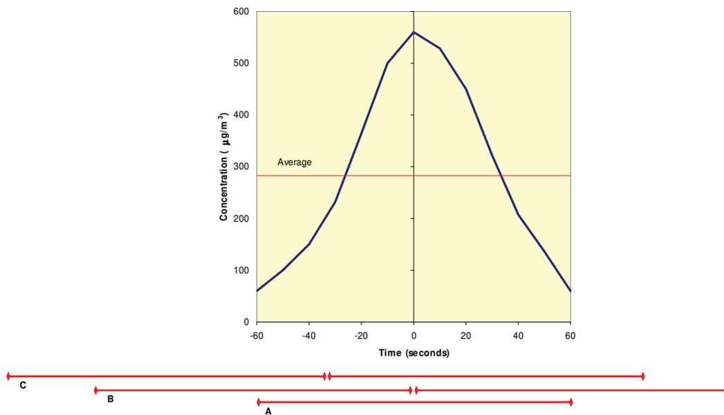
**Figure 4: Nitrogen Oxides Peak Shape and Examples of Different 2-minute Averaging Periods. Lines A to C Discussed in the Text.**
