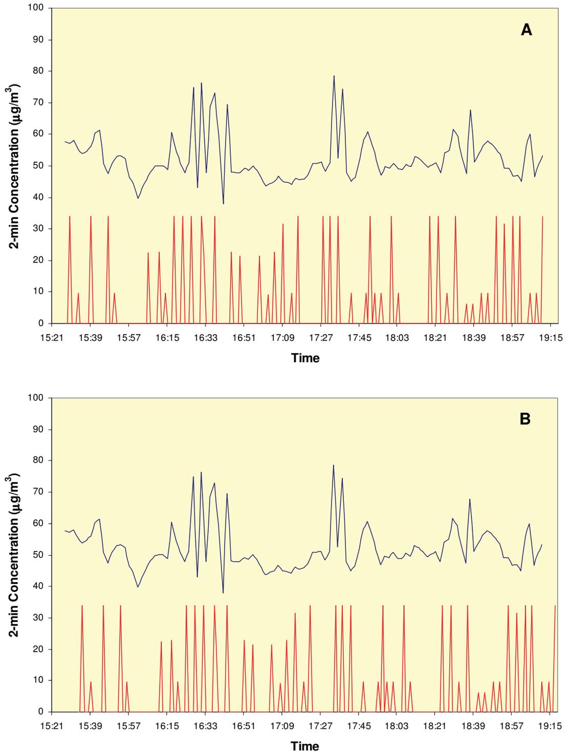
**Figure 10** Measured (blue line) and Simulated (red line) Nitrogen Oxides Concentrations (maxima) at the London City Airport Newham Docklands Monitoring Site on the Morning of 12 December 2008. A = times as recorded. B = 10 minute time shift in Aircraft Peaks
