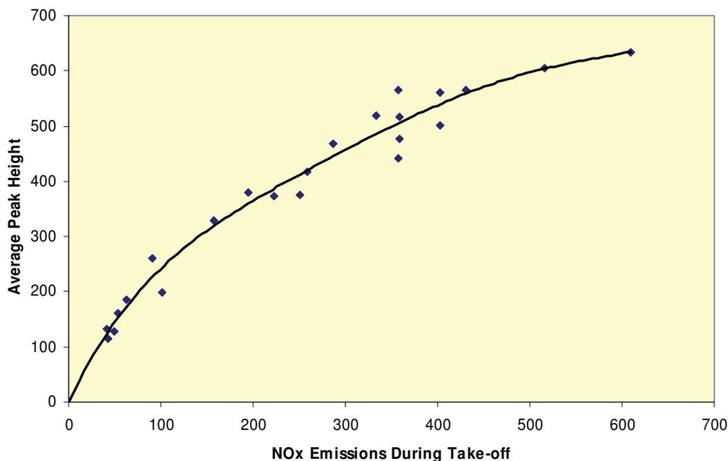
**Figure 3: Relationship Between Average NOx Peak Height (µg/m<sup>3</sup>) and NOx Emissions During Take-Off (g/s) at Heathrow Airport**
