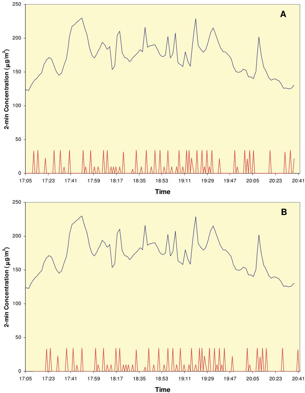
**Figure 9 Measured (blue line) and Simulated (red line) Nitrogen Oxides Concentrations (maxima) at the London City Airport Newham Docklands Monitoring Site on the Morning of 29 October 2008. A = times as recorded. B = 10 minute time shift in aircraft peaks**
