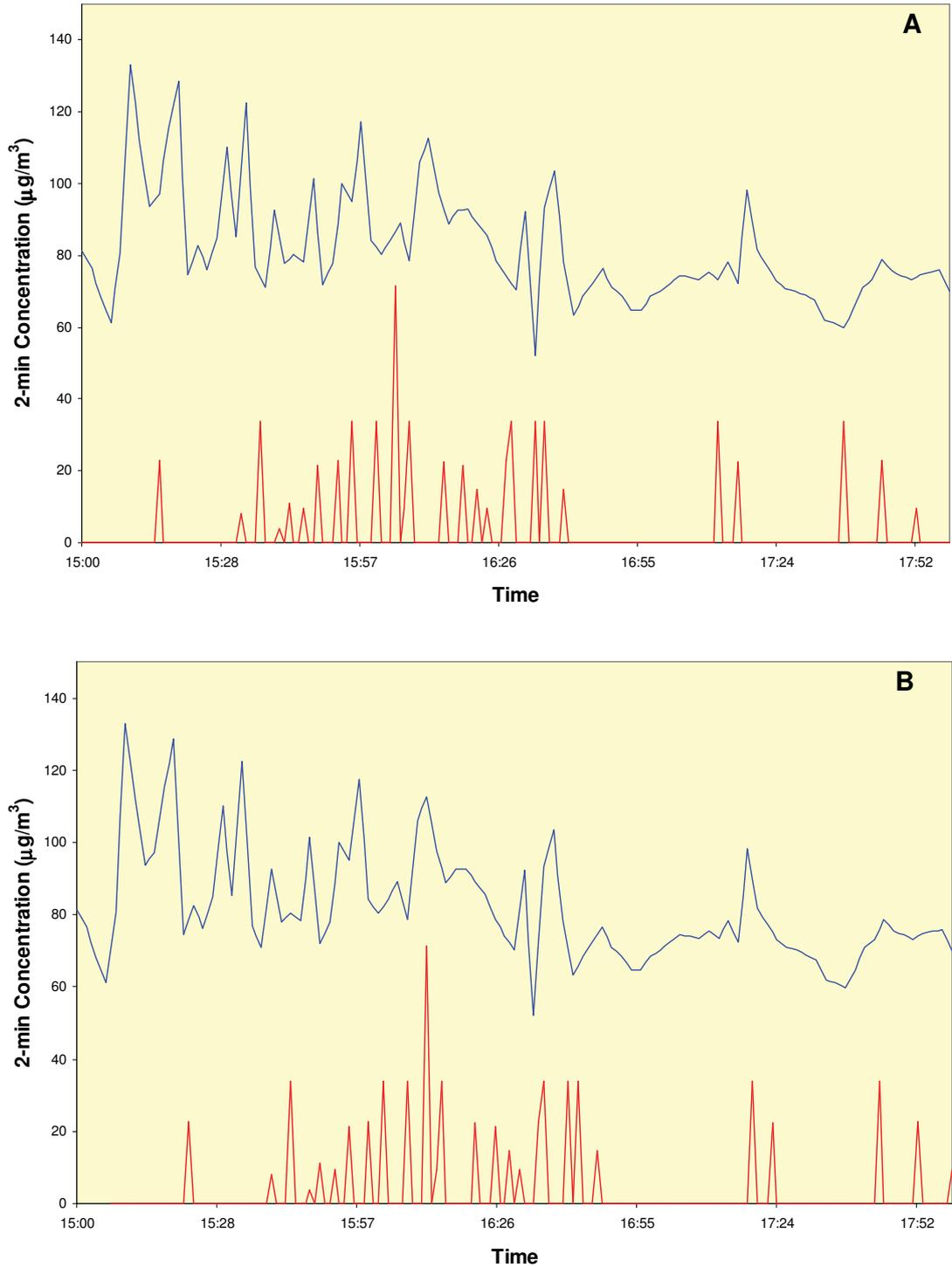
**Figure 12 Measured (blue line) and Simulated (red line) Nitrogen Oxides Concentrations (maxima) at the London City Airport Newham Docklands Monitoring Site on the Afternoon of 12 November 2009. A = times as recorded; B = 7 minute time shift in Aircraft Peaks**
