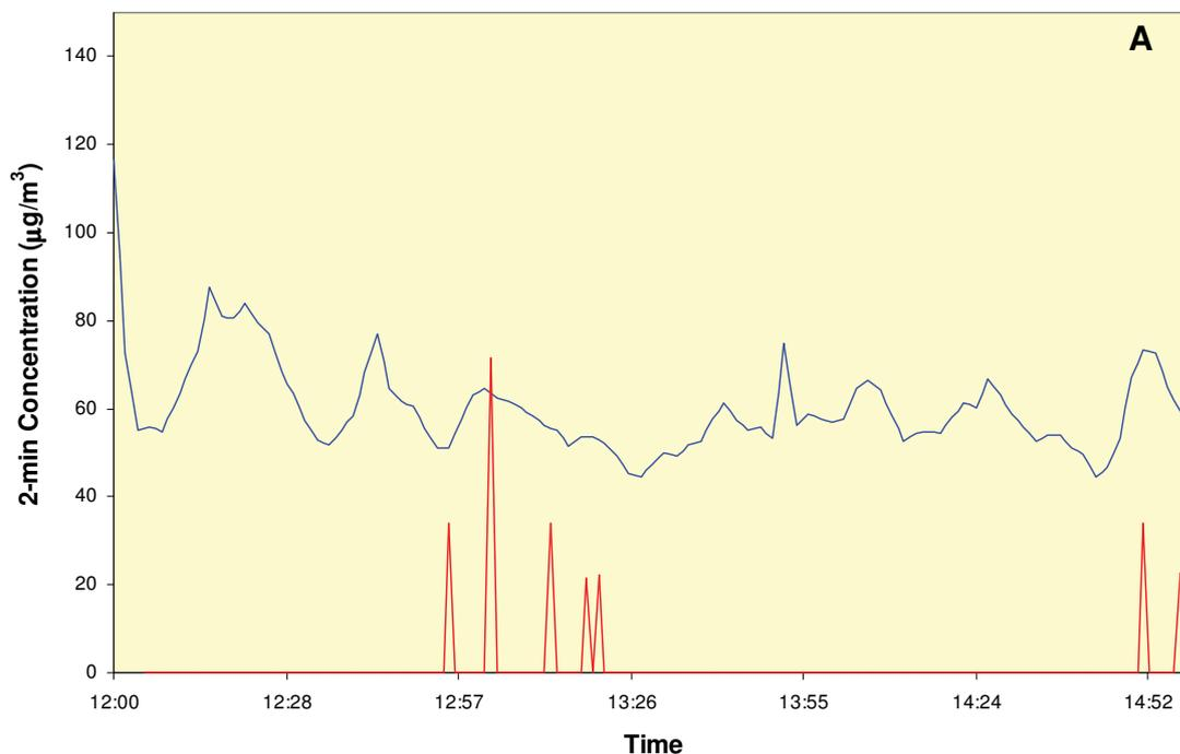
**Figure 13** Measured (blue line) and Simulated (red line) Nitrogen Oxides Concentrations (maxima) at the London City Airport Newham Docklands Monitoring Site on the afternoon of 19 October 2009.
