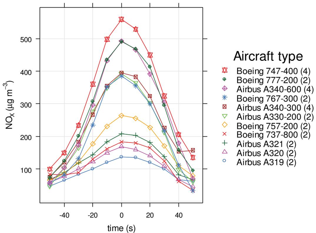
**Figure 2: Average 10-Second Nitrogen Oxides Concentrations for Different Aircraft Types at LHR2 Monitoring Site at Heathrow Airport**
