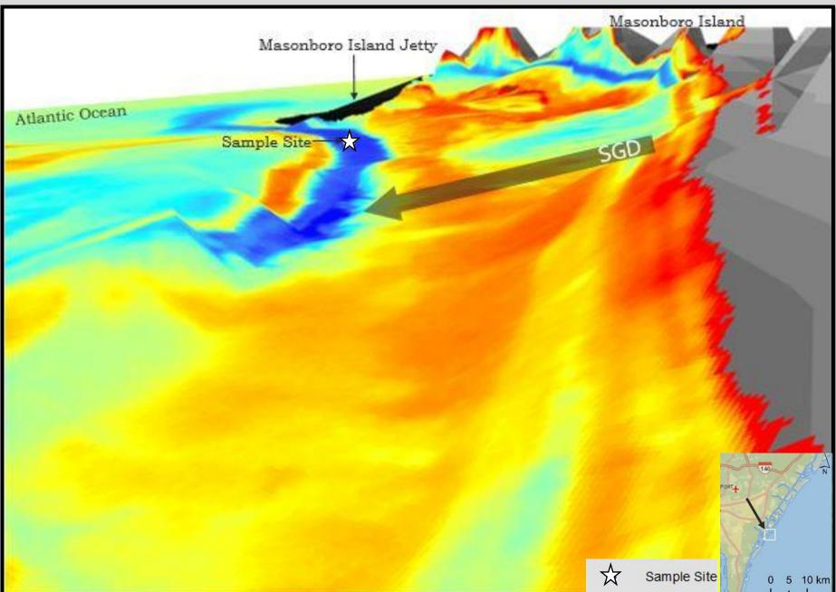
Off-Nadir view of Masonboro Island UAS-TIR Survey region water surface to enable hydrologic gradient and SGD flux to be modeled 226Ra = 0.09 dpm/L Sandy Sediments  $\phi = 0.9$ <sup>26</sup>Ra = 1.8 dpm/L  $\tau = 0.4 vr$ Leaky Confining Layer Limestone  $\phi = 0.5$ 26Ra = 9 dpm/L <sup>222</sup>Rn Decay Chain: <sup>226</sup>Ra emanation from sediments to <sup>222</sup>Rn,
