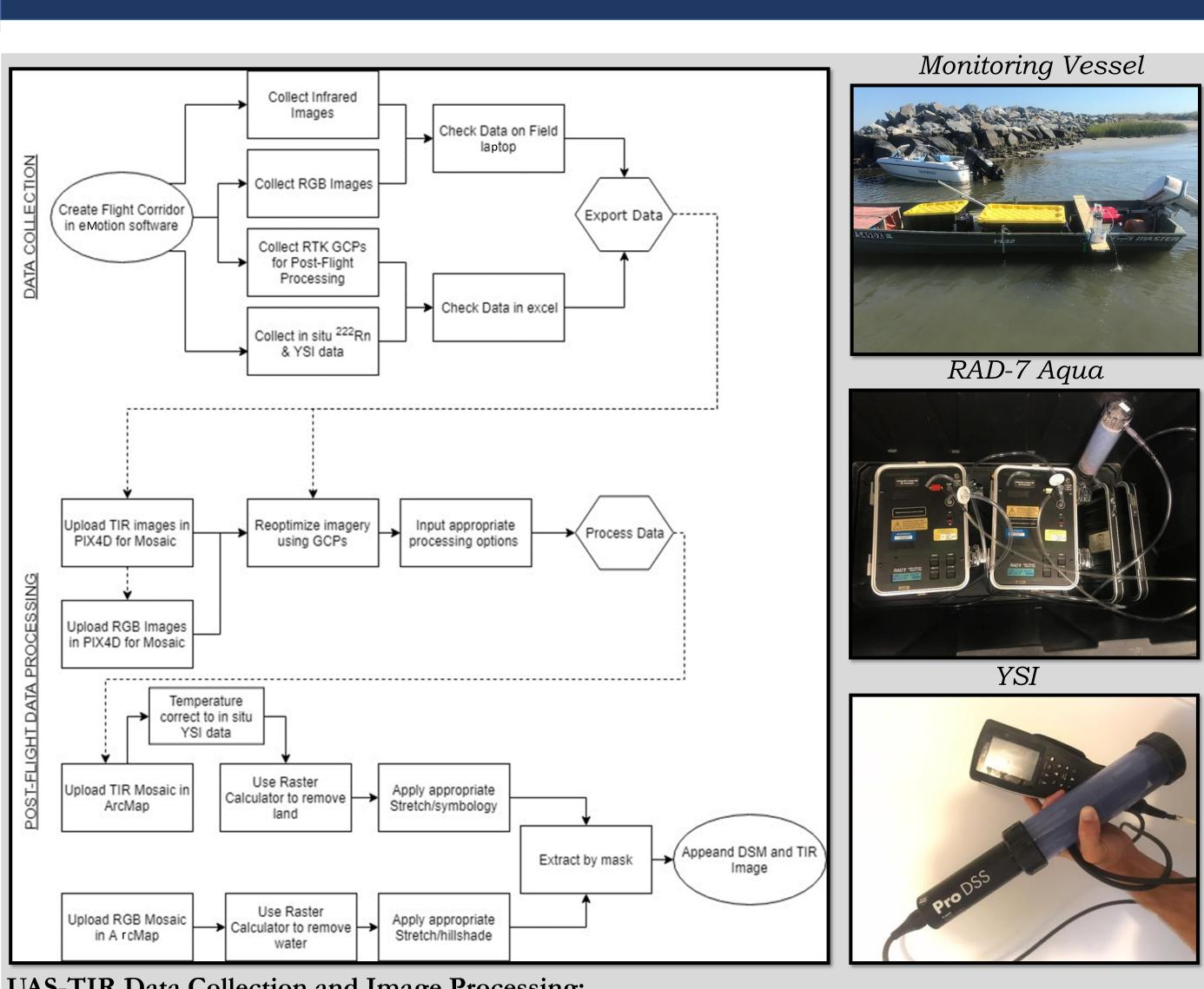
**UAS-TIR Data Collection and Image Processing:** Accurate orthomosaics (maps) of UAS-TIR data at prominent SGD plumes were produced using an eBee professional drone equipped with a high-resolution senseFly thermoMap sensor, capable of detecting 0.1°C at approximately 14 cm/pixel. Multiple flights were required to image the entire region of interest because UAS battery life. FAA regulations require all flights to be below an altitude of 122 meters. **Radon Time Series Measurements:**
