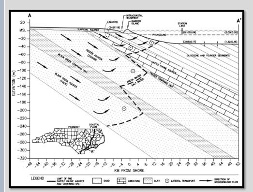
**Geology:** Stratigraphic cross section of geology, aquifers and SGD flow in study region <sup>5</sup>
