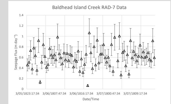
Estimated seepage rates over the experimental period based on the radon model and using a pore water radon concentration of 1000 Bq m<sup>-3</sup>. Error bars above and below the SGD estimates (open *triangles) represent ±25% uncertainties.*
