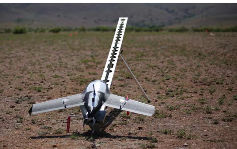
Figure 8. Trimble Gatewing X100 on the catapult in Mexico.
