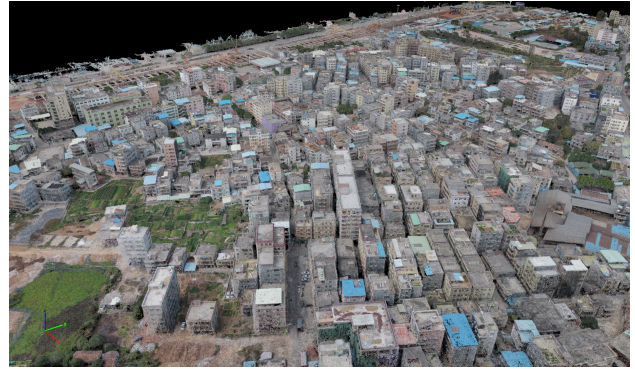
Figure 11. Large data set reconstruction using Pix4Dmapper 2.1. It was created from 1700 images captured in several flights using a DJI Phantom 2 Vision+. It covers an area of half a square kilometer with a ground sampling distance of 3.4 cm.
