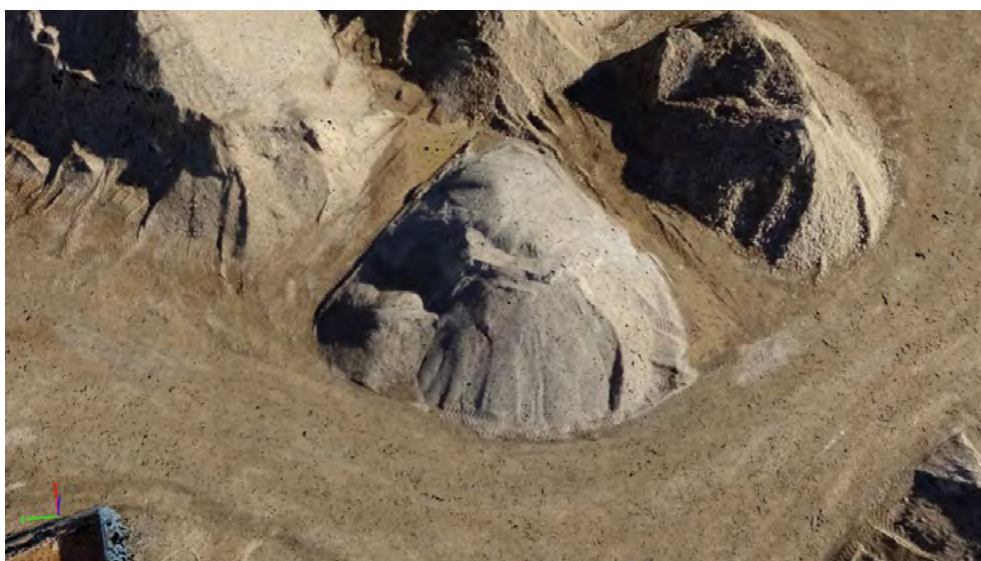
Standard stockpiles may be roughly conical in shape. Data set source: courtesy of Geomatic Development
