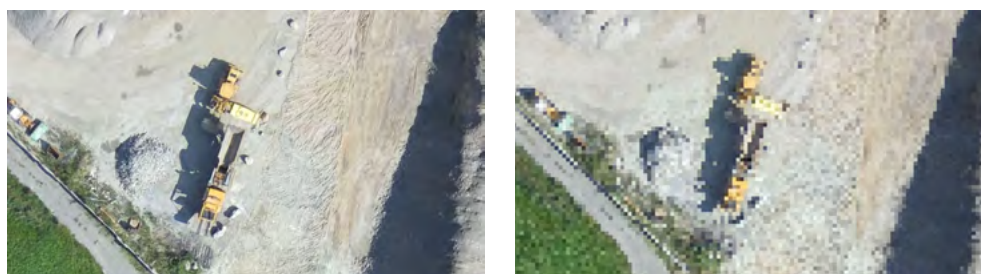
The image on the left has a GSD of 5cm, and the image on the right has a GSD of 30cm
