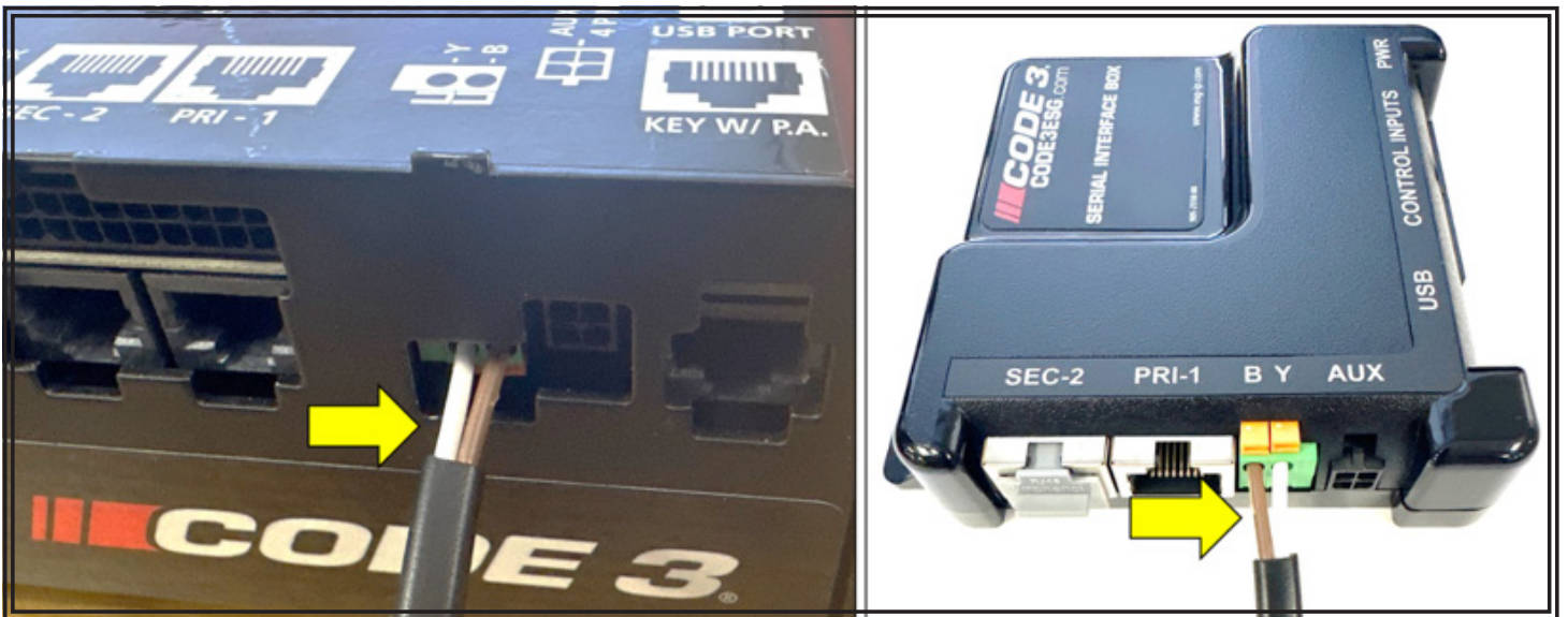
Figure 2 Connecting 690-1111-02 to a SIB or Z3
