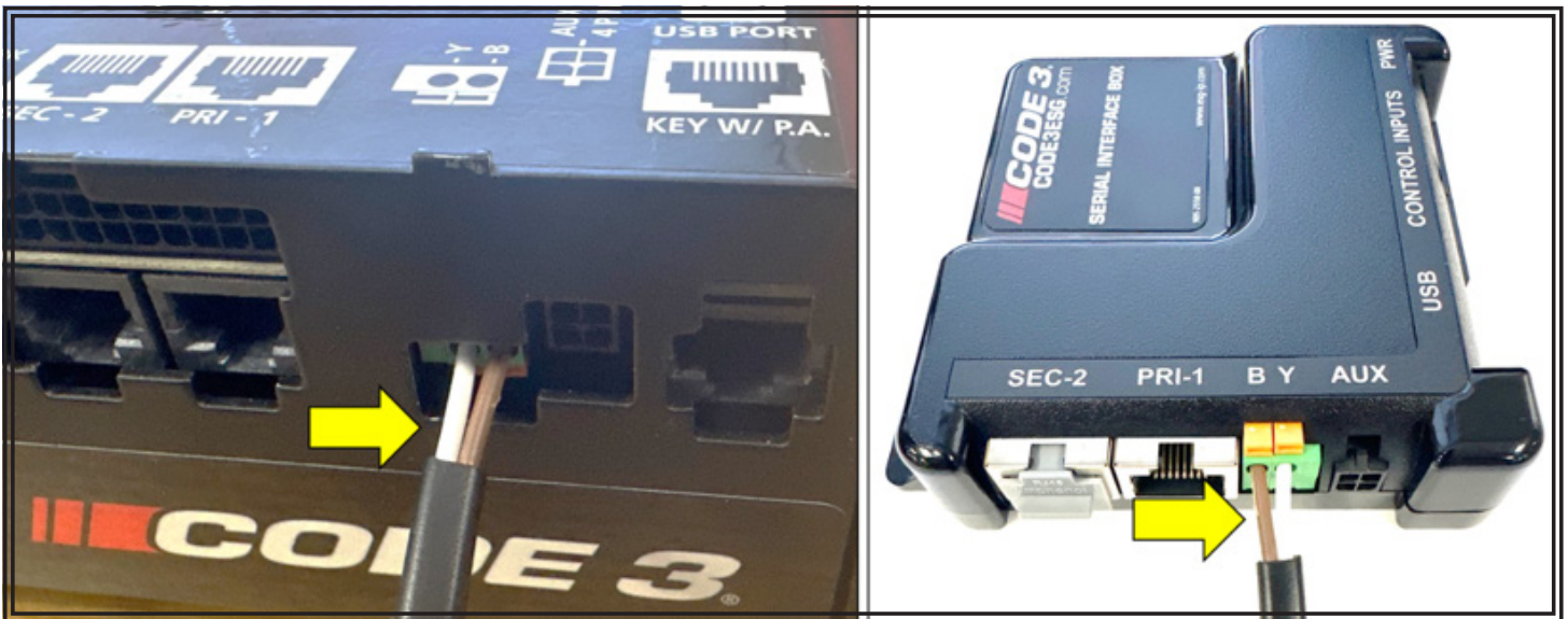
Figure 2 Connecting 690-1111-02 to a SIB or Z3
