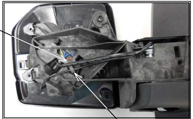
Figure-6 ZIP TIE WIRING CONNECTIONS TO THIS WIRING RETENTION TAB.
