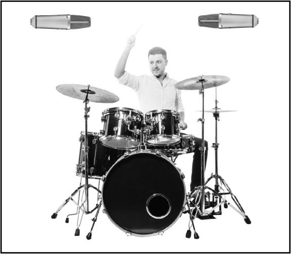
In this diagram, two WA-67's are used in a spaced pair configuration to record stereo drum overheads.
