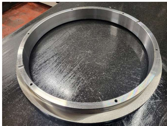
Figure 404: Sealing ring for rotors [UK]
