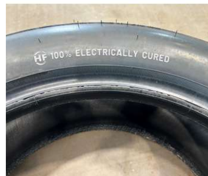
Figure 28: Electrically cured tyre
