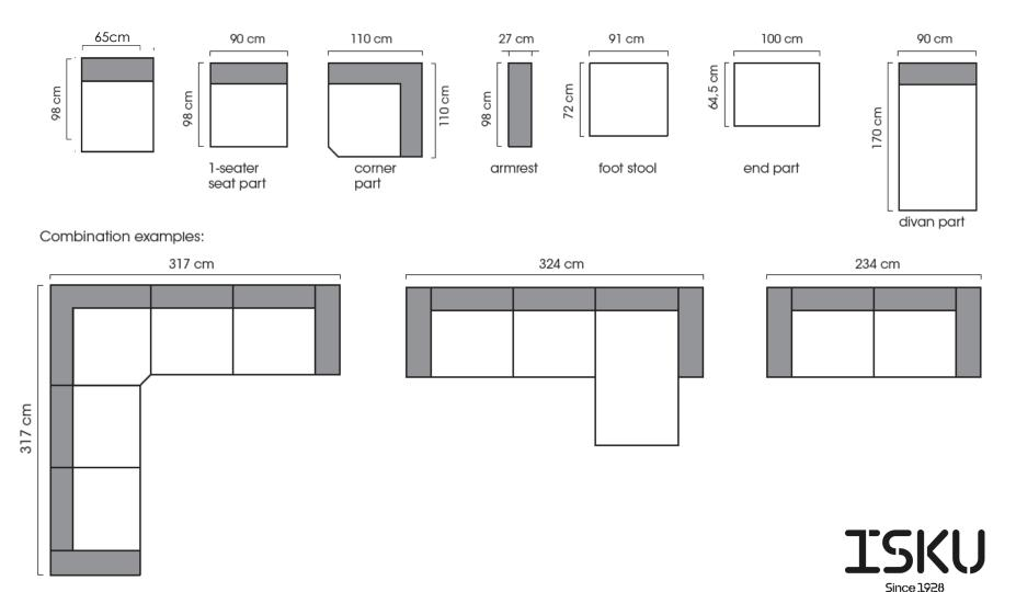
Dimensions depend on the selected modules. The height of all modules with backrest is 770 mm- The seating height of all modules is 470 mm.
