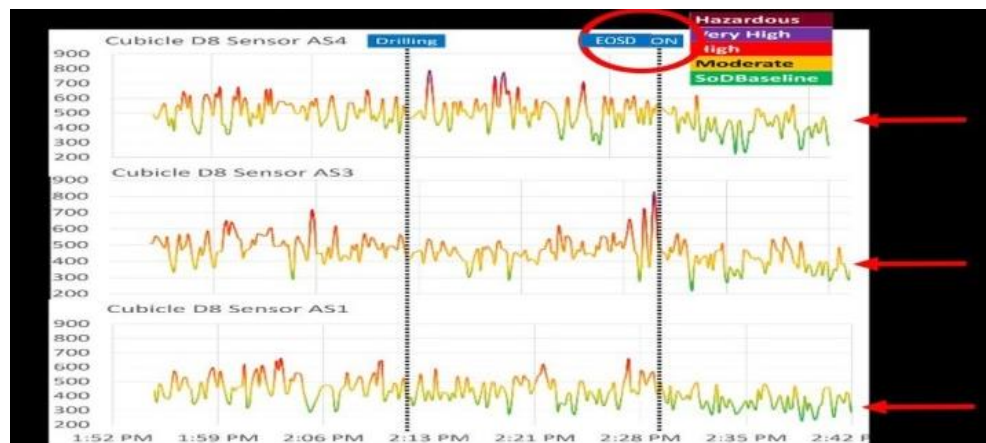
Figure 4: Even with the operation of EOSD, there are peaks of red (high particulates) above the green background level, which means that aerosols (particulates) are escaping.
