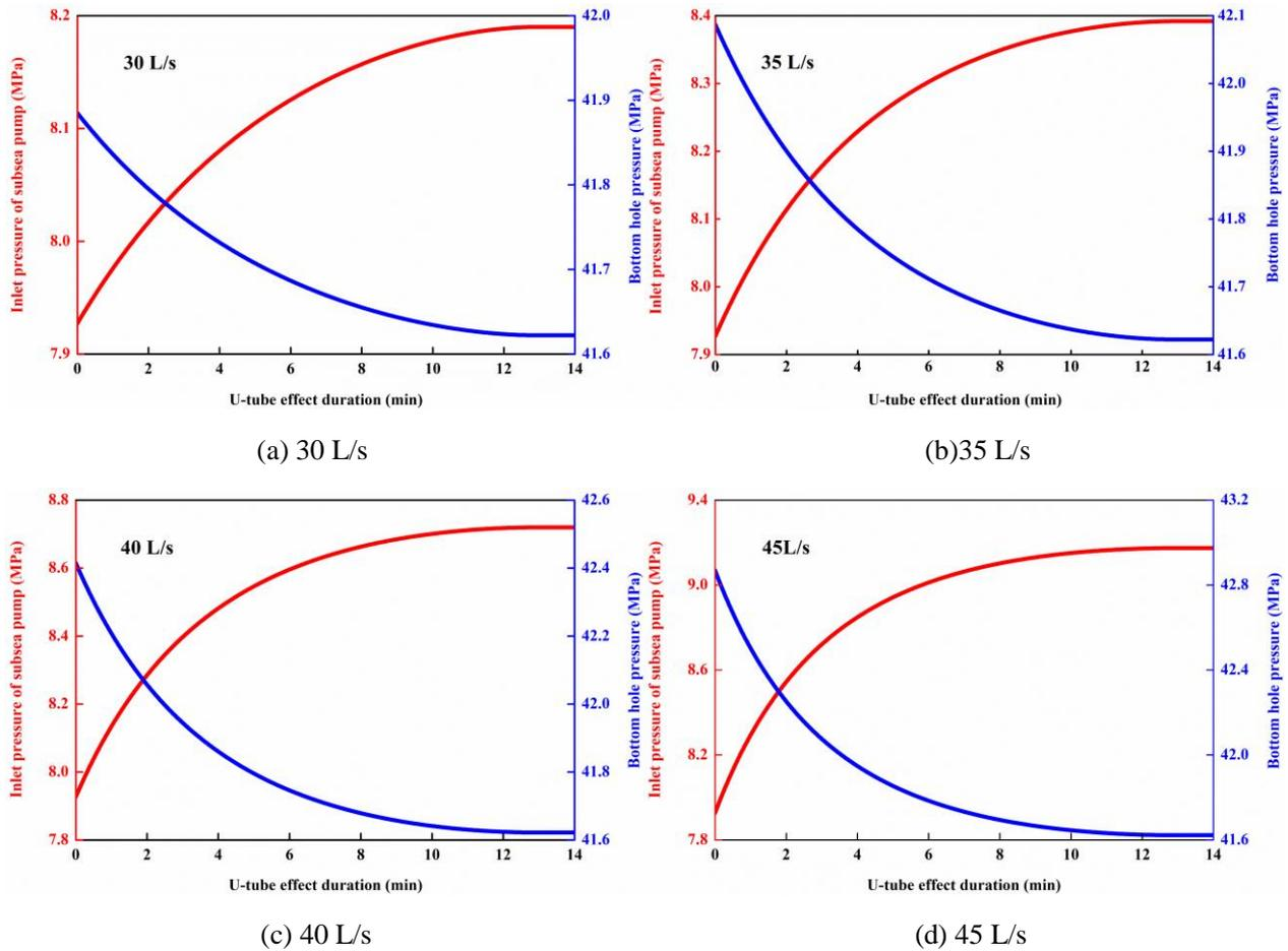
**Figure 4:** The relationship between the inlet pressure of the subsea pump and the bottom hole pressure under different drilling pump displacements before shutting down
