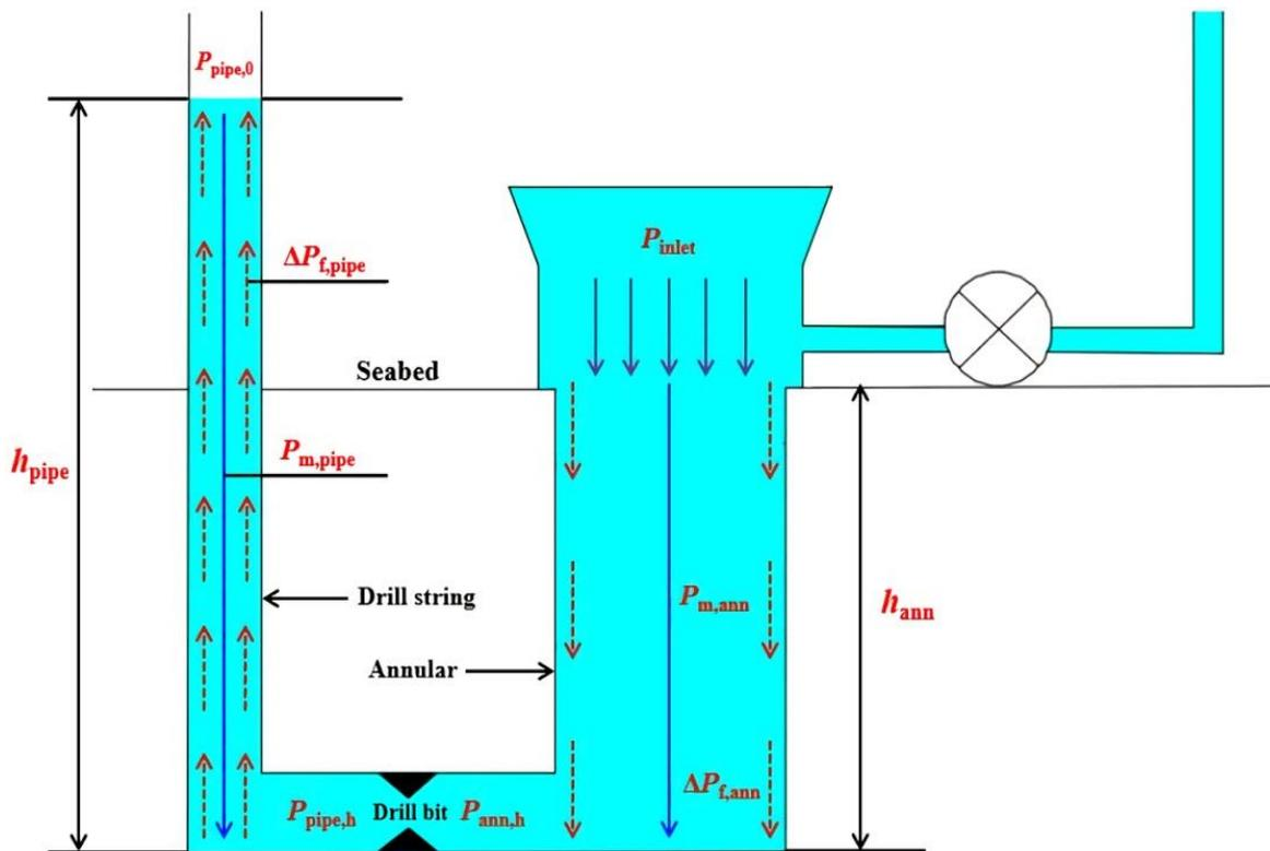
Figure 1: Physical model of annulus pressure distribution when drilling pump is shutdown
