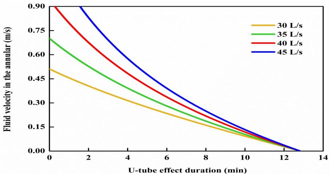
Figure 2: Changes of fluid return velocity in annulus of RMR system during U-tube effect
