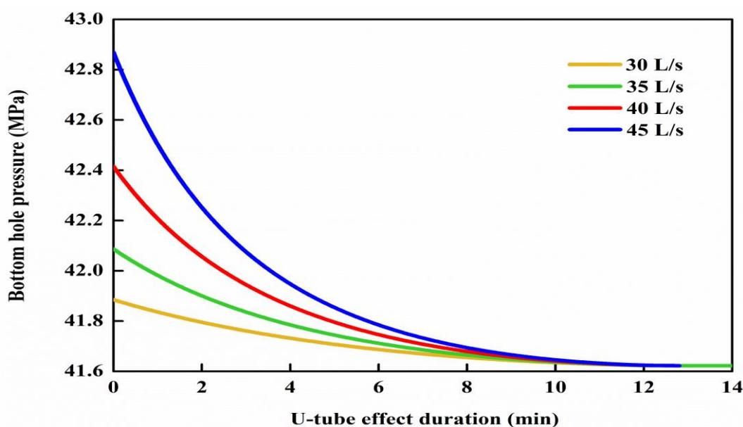
Figure 3: Changes of bottom hole pressure of RMR system during U-tube effect
