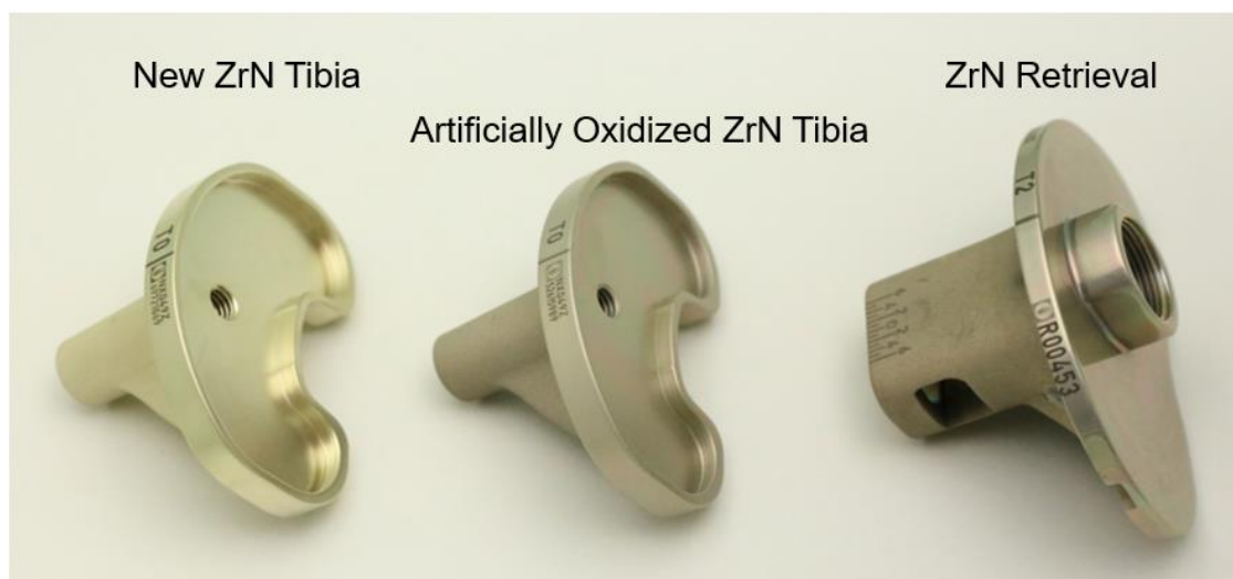
Figure 4: Color change comparison between a new out of the box ZrN tibial component, an artificially oxidized ZrN tibial component and a ZrN retrieval with surface oxidation.
