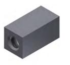
Square Nuts with low heights are used as counter nuts in order to achieve a slip-free bar connection despite the coarse thread. They are only designed for transferring the counter moment and cannot be used as anchor nuts.
