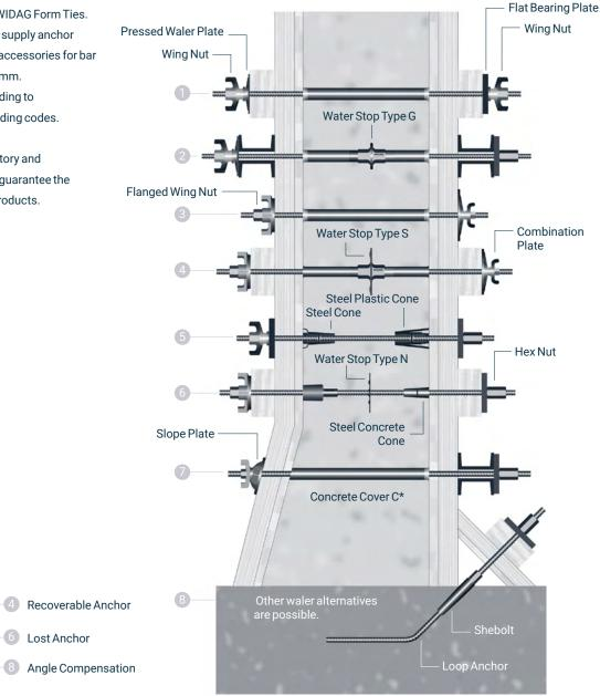
\* Length of Lost Anchor = Wall Thickness -  $2 ext{ x Concrete Cover C}$
