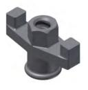
With different Waler Plates, Wing Nuts can be used as anchor nuts both for timber and steel walings. They can be fixed and loosened using a hexagon wrench or a threadbar.
