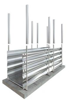
Step 4 Stabilize the width of formwork with S-hook
