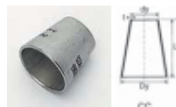
ISO, EN1.4307/304L (SS2352) EN10253-3 CC. L=3 x (Dy-dy).
