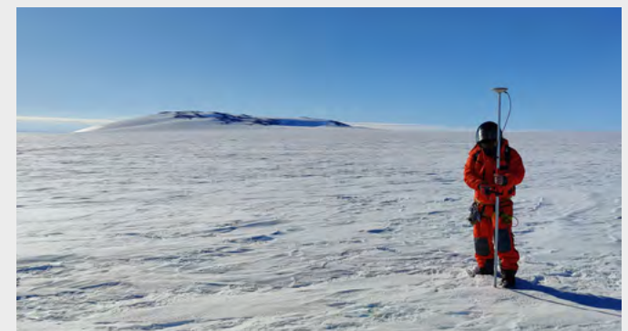
Jyri measuring the height of the glacier with RTK-GPS. Photo: Arttu Raja-Halli
