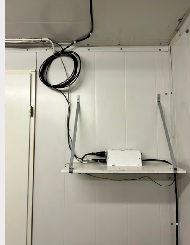
Nanometrics Centaur digitizer in an absolute gravimetry container in Aboa. Photo: Priit Tisler / FINNARP
