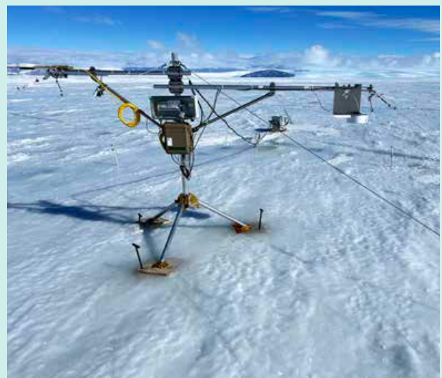
Mini-radiation station installed on NIS from 30.11.2025 to 22.01.2026. The station was 70 m apart the bigger AWS and measured the surface net radiation budget and the surface spectral albedo.
