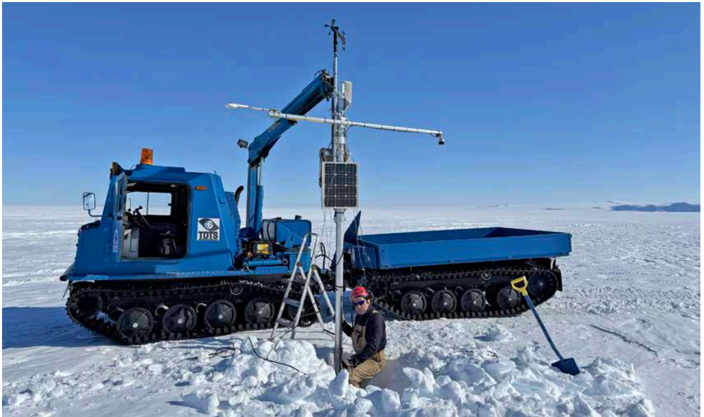
Priit Tisler maintaining the AWS5 automatic weather station on the glacier. The annual snow accumulation averages 40–60 cm.
