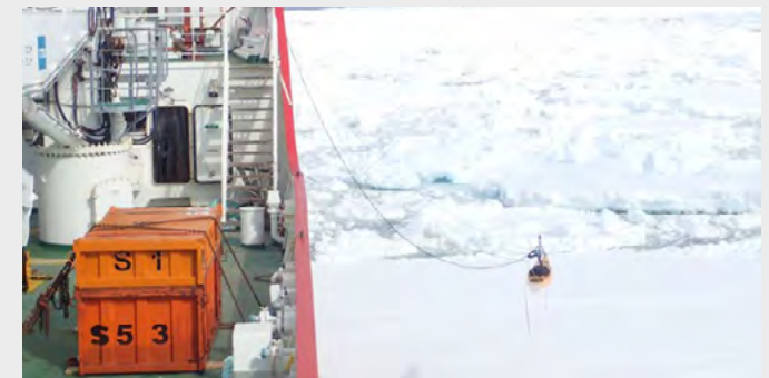
Electromagnetic sounder inside the kayak measuring sea ice thickness. Photo: Jaakko Seppänen
