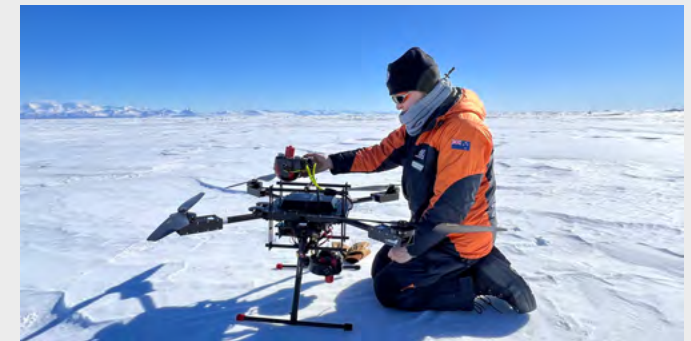
Drone Spectra equipped with upward and downward-looking Kipp and Zonen CM4 pyranometers and Ocean Optics STS VIS and NIR spectro-radiometers for broadband and spectral albedo measurements. Photo: J. Martin
