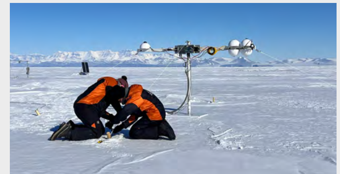
Broadband radiation station powered with solar panels. Photo: J. Martin
