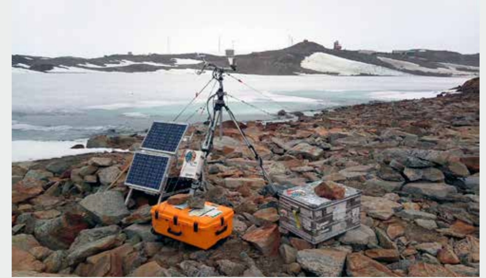
Eddy-covariance mittauksia Glubokoe järven rannalla. The eddy covariance tower deployed on the coast of the Lake Glubokoe. Kuva | Photo: Elena Shevnina
