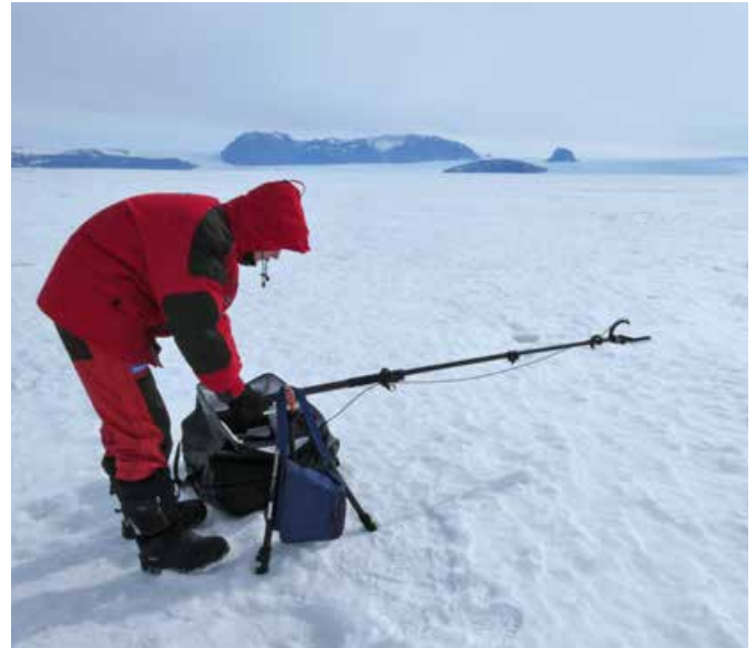
Anja Mödl measuring the surface spectral albedo along a transect with the portable ASD FieldSpec radiometer.
