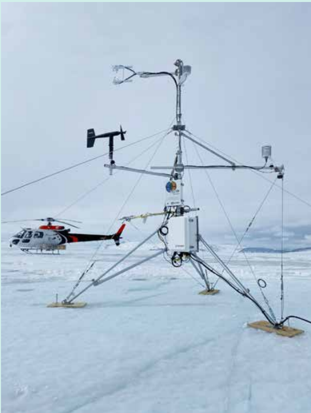
FMI Automatic weather station installed on NIS from 28.11.2025 to 22.01.2026. The station measured the net surface radiation budget, the 2m temperature, humidity, wind speed and direction, the 3.5m turbulent fluxes, water vapor flux, temperature and humidity, as well as the snow depth.
