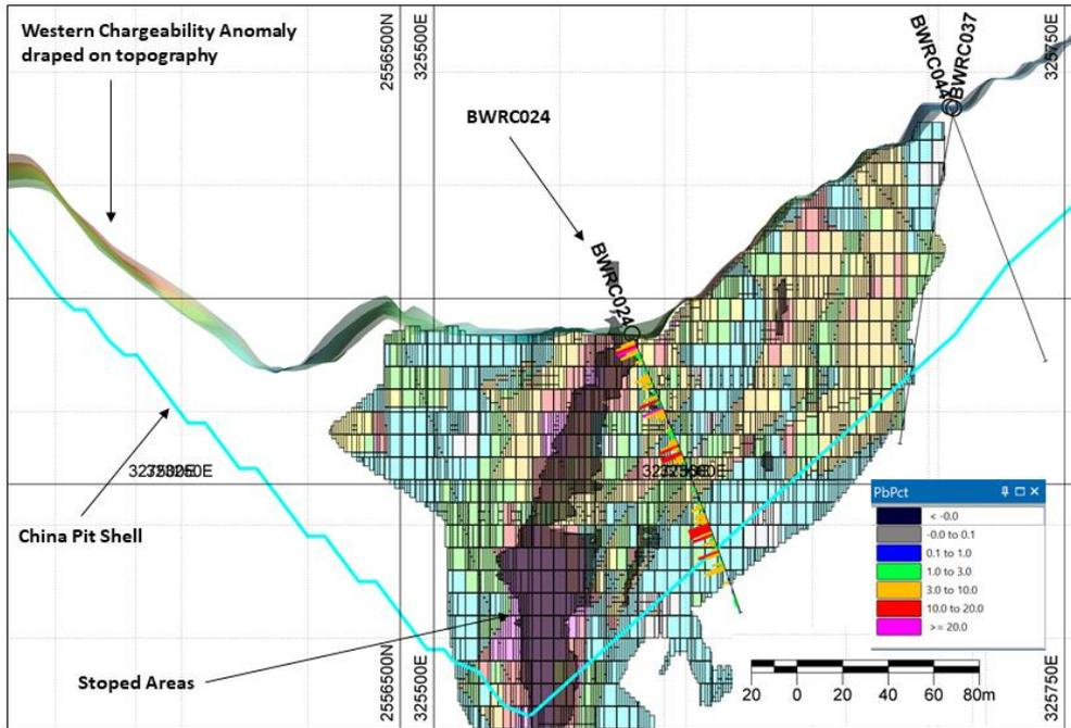
Figure 3. Section showing BWRC024, drilled into China Lode (looking northwest) with block model and drill traces coloured for lead grade. The hole verified the positions of the modelled high-grade lodes as well as intersecting a new high-grade zone at depth.
