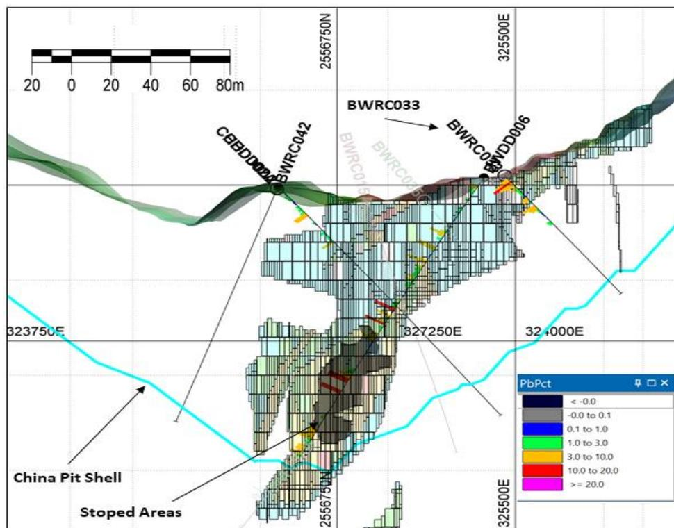
Figure 4. Section showing BWRC033, drilled into China Lode (looking northwest) with block model and drill traces coloured for lead grade. The hole verified the positions of the modelled lead and copper mineralisation which was based on historic underground channel samples
