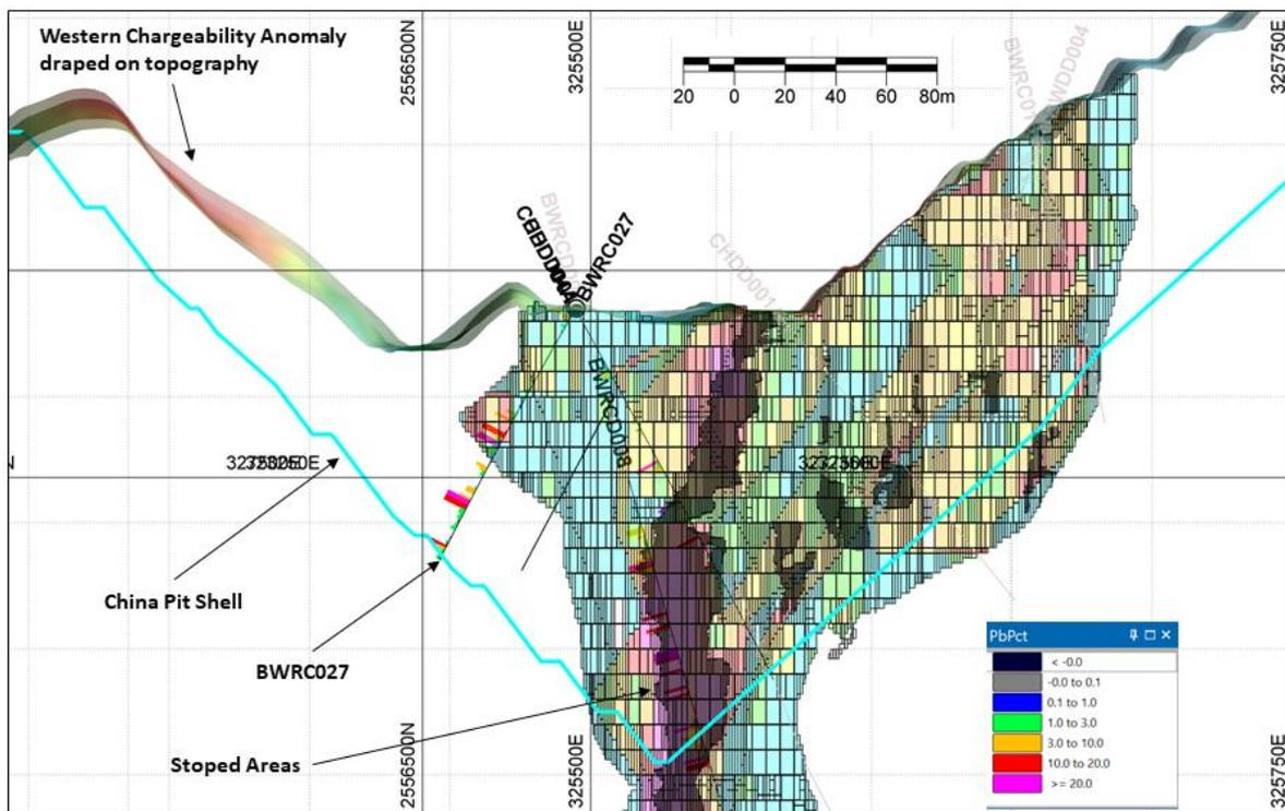
Figure 2. Cross section (looking northwest) showing location of BWRC027 infilling between China Resource block model and current pit shell. Of interest is a chargeability anomaly on the hill near the western boundary of the pit shell.
