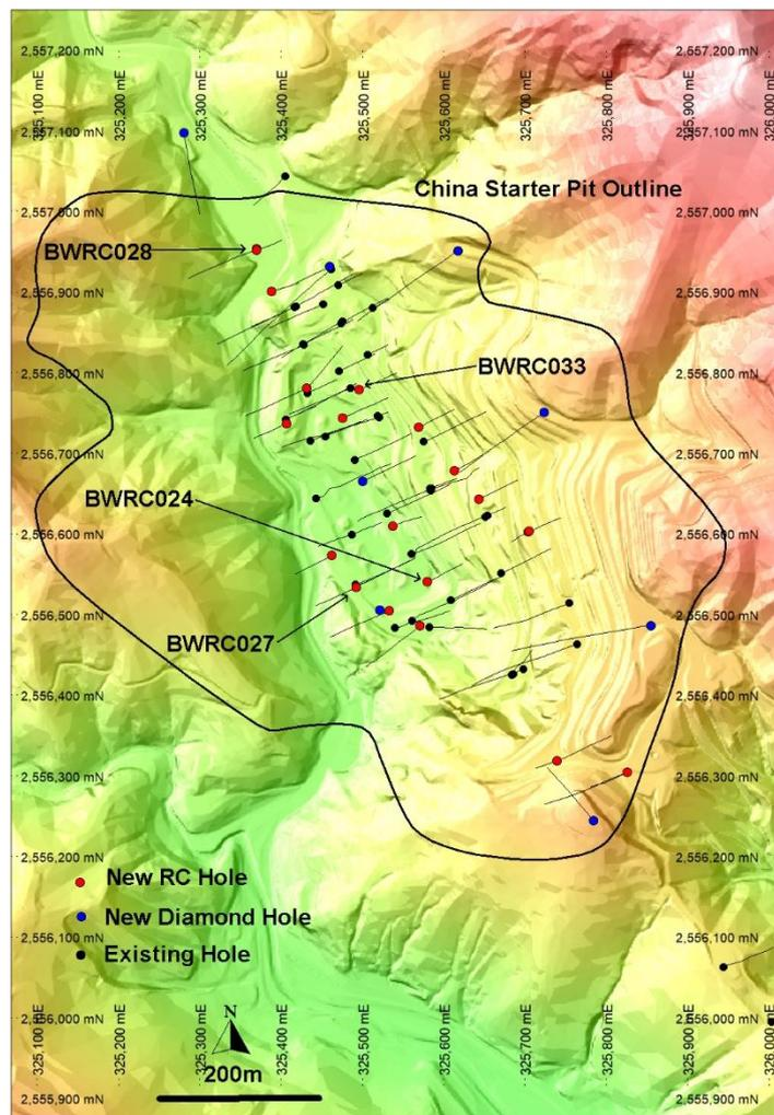
Figure 1. Drilling locations on topography.
