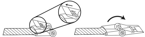
**A. To open ratchet all the way, pull up on the spring-loaded bar.**
