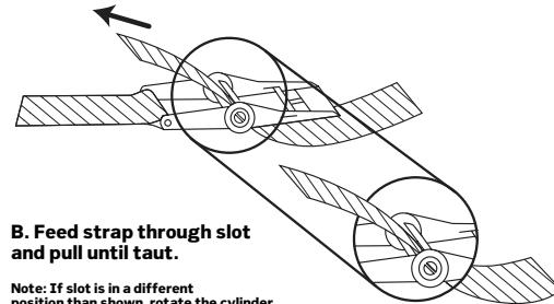
**B. Feed strap through slot and pull until taut.**
