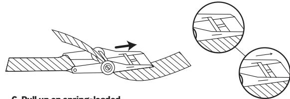
**C. Pull up on spring-loaded bar to close the ratchet.**
