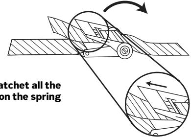
**A. To open ratchet all the way, pull up on the spring loaded bar.**
