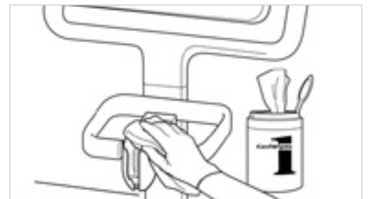
Figure 6: Remove gross contaminants on the cradle using CaviWipes1
