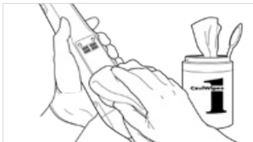
Figure 3: Remove gross contaminants using CaviWipes 1
