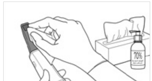
Figure 5: Wipe the optical surface of the wand with IPA
