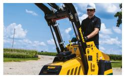
**ISO-RATED OPERATING CAPACITY** for the S725TX is 750 lbs (340.2 kg). With a rated tipping load of 2145 lbs (973 kg), this small footprint machine positions itself as an exceptional mini skid steer. Additionally, the S725TX leads the industry with a lift height (to hinge pin) of 84.5" (214.6 cm).
