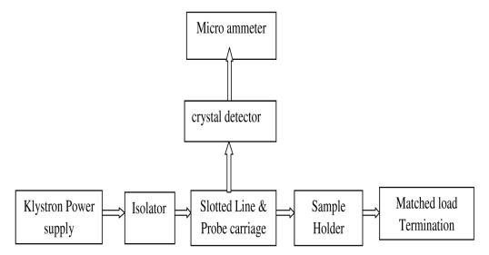
Fig (i) Block Diagram of the Experimental Setup
