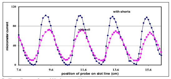
fig (ii)standing waveform within the waveguide
