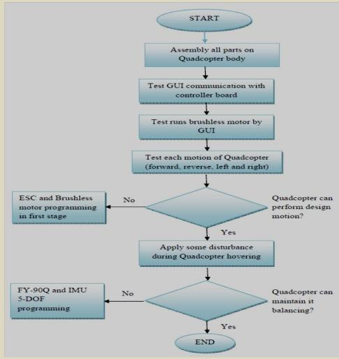
Figure 3: Flow chart of quad-copter design
