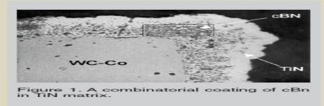
Fig: Nanocomposite Coating
