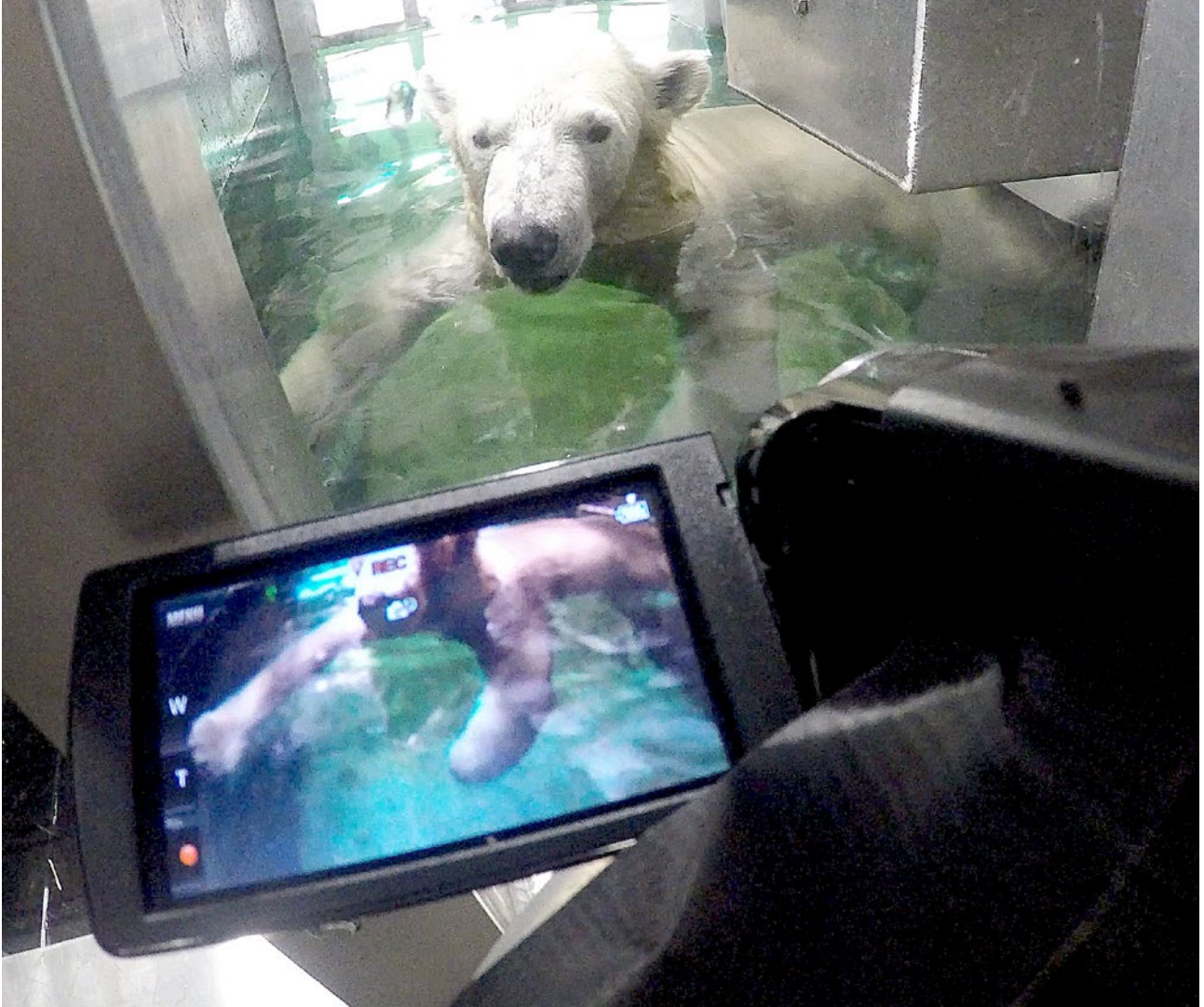
A swim flume chamber, built to measure the bear's oxygen consumption as it swims at different speeds. Photo courtesy of Michael Durham / Oregon Zoo.
