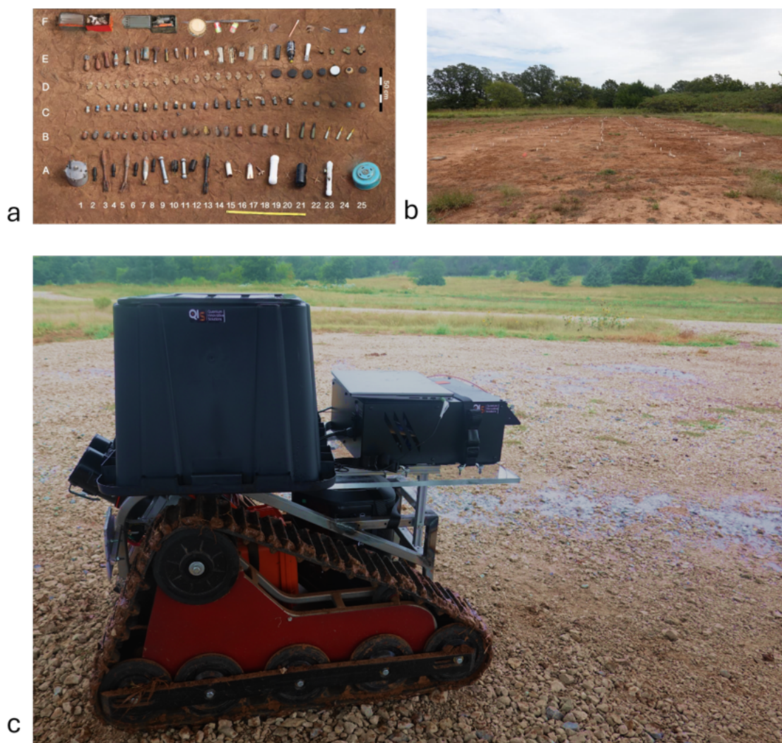
Figure 3: portrays the testing range at CENFEX: a) Depicts 143 mine types buried at various depths. b) Shows the range with inert landmines ready for measurement. c) Illustrates the vibrometer integrated with the ground rover.
