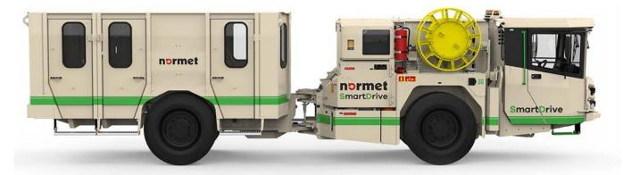
Utimec MF 205 PER SD with 20+2 persons transport capacity is designed for people transportation in underground mines and tunnels. Utimec personnel carrier includes several safety features as standard. Vehicle has an front axle suspension system or optional full chassis suspension which improve safety, driving comfort, passenger ergonomics and increases component lifetime
