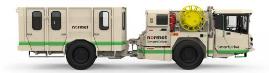
Utimec MF 205 PER SD with 20+2 persons transport capacity is designed for people transportation in underground mines and tunnels. Utimec personnel carrier includes several safety features as standard. Vehicle has an front axle suspension system or optional full chassis suspension which improve safety, driving comfort, passenger ergonomics and increases component lifetime
