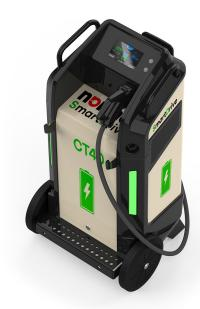
Normet SmartDrive CT40 is state-of-the-art Finnish DC-charging trolley, which is tailor made for harsh underground conditions. The trolley does not require permanent installation and it is an ideal mobile charger for workshops and service depots. It is compatible with the CCS charging communication standard and equipped with one or two fast charging plugs (Type 2), offering output power of 40 kW.
