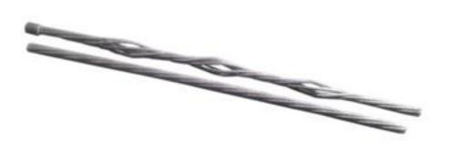
The cable bolt is a seven wire strand nominally 21.6 mm diameter cable without bulbs, and can be with grout or resin encapsulated. A central king wire is surrounded by six wires of similar diameter (7.4 mm), with a lay of approximately 320 mm, which have been cut with a spiral indent of 2.5 mm wide.
