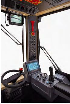
Electric system is designed for harsh underground environment. System consists of self-extinguishing wire harnesses with tinned wires, water tight conduits and all exposed components are minimum IP65 protection class. In addition, vehicle layout allows easy access to all service points, all daily checks can be done from the ground level.
