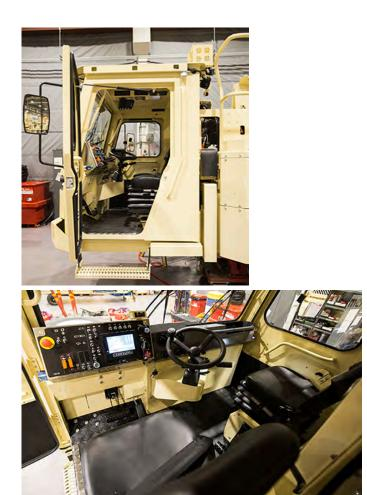
NorSmart 2 electric system is designed for harsh underground environment. System consists of self-extinguishing wire harnesses with tinned wires, water tight conduits and all exposed components are minimum IP65 protection class. In addition, vehicle layout allows easy access to all service points, all daily checks can be done from the ground level.
