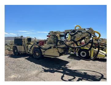
Spraymec is equipped with new SB500-B Boom assembly
