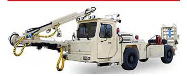
Agile charging manipulator boom is easy and fast to operate and has kinematics and reach to operate full 360-degree stoping round. Foldable telescopic boom structure enables to pick primer from ground and erect it to upholes without need of climb on top of boulders exposing operators to accidents.
