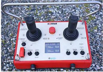
Charging boom radio control and open load end to accommodate up to 6-ton total weight bulk emulsion systems enables highest productivity and operating safety.
